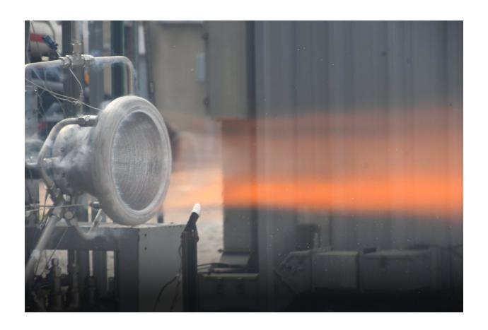
The RAMFIRE nozzle performs a hot fire test at Marshall's East test area stand 115. The nozzle, made of the novel aluminum alloy 6061-RAM2, experiences huge temperature gradients. As hot gasses approach 6,000° Fahrenheit and undergo combustion, icicles are forming on the outside of the engine nozzle. Credit: NASA
